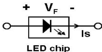
**Note 4-2:**  $\Delta V_s (\text{Max.}) = \Delta V_F \times \text{LED No. (one string)}$ ;
